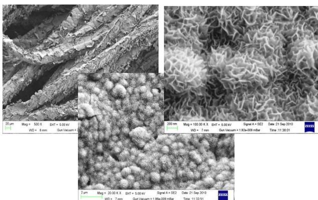
Biom mineralized chitosan-TPP fibers
