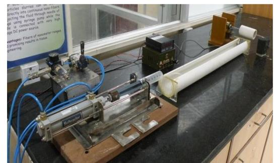
**Laboratory scale wet spinning setup**
