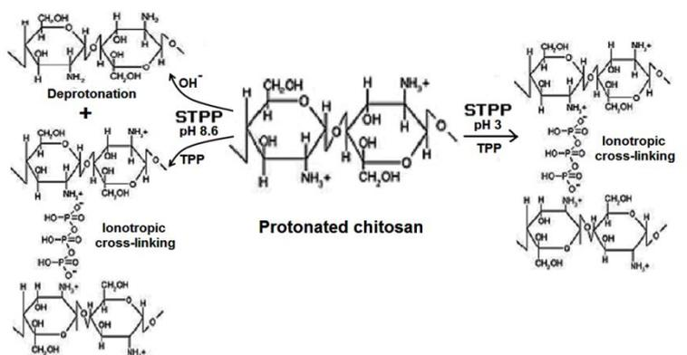
Gelation mechanism of chitosan in STPP solution at pH 3 and 8.6
